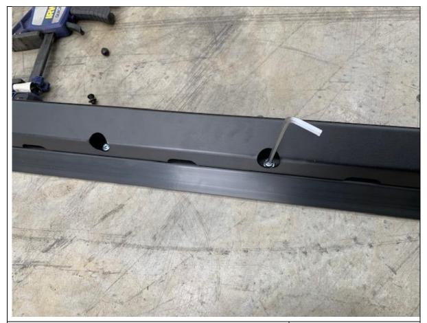
27. Thread cap screws into each hole
