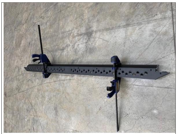
28. Flip entire slider up as shown29. Clamp step hard to extrusion
