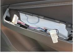
• To remove the connectors from the underside of the switch assembly, push the tabs inwards and then remove.
