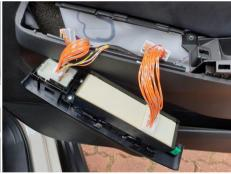
Position the window switch fascia front end first so it engages the locating lug and lower back into place
