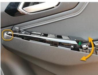
The switch fascia assembly can now be pulled out and turned upside down to gain access to the two connectors
