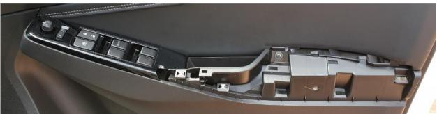
• Remove any clips left in the door panel and place back into position on the armrest.
