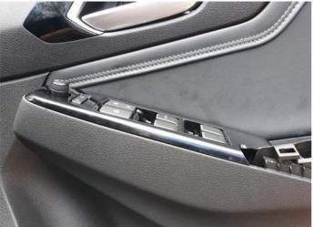
• Ensure all cables and connectors are not positioned to obstruct the switch assembly from fitting correctly, if any obstructions are placed on the switch connectors this may affect the operation of the switches.
