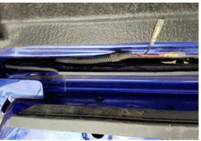
Select where you want to have it enter into the tail gate, I used the very first opening, then into the main area of the tail gate.
