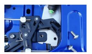
Align the holes within the stainless steel bracket to the latch and lock threads, refit the Torx bolt to the lock mechanism first, do not fully tighten.
