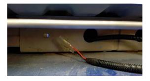
**NOTE:** If you have the factory camera fitted, you can use the existing entry point through the grommet, you will need to remove a section of the split tubing before passing the cable through, and then refit the spit tubing once inside the tailgate.
