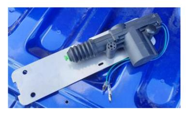
Fit the actuator using the 2 provided screws to the supplied stainless steel bracket in the orientation shown above.
