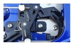
Using the supplied 3mm hex shaft drill bit in an cordless drill or impact driver, drill a 3mm hole in the centre of the plastic latch assembly that you have just marked.
