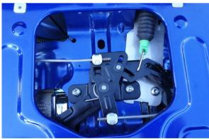
Connect the harness to the actuator wires by pushing the corresponding bullet terminals together firmly.
