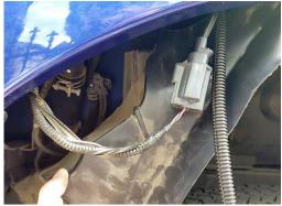
Run the harness down on the right-hand side of the fuel inlet hose so it exits on the other side.
