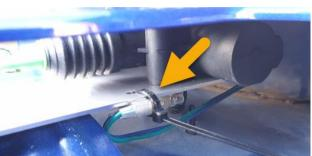
Refit tail gate trim; reinsert all plastic plugs that had been removed from the rear inner guard during the installation process.
