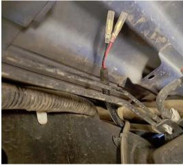
Then follow the existing cables back to the rear of the car, using the supplied cable ties to hold it in place.
